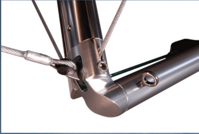
VG cord routing is down the centre of the aluminium upright tube. This makes the VG cord light to pull. Centre routing also makes changing the VG upright easy.
