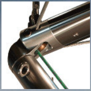
VG cord routing is down the centre of the aluminium upright tube. This makes the VG cord light to pull. Centre routing also makes changing the VG upright easy.
